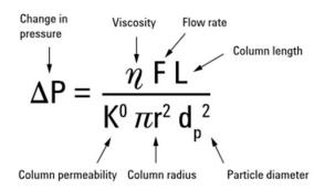
As the particle diameter is decreased by a factor of two, the backpressure goes up by a factor of four
