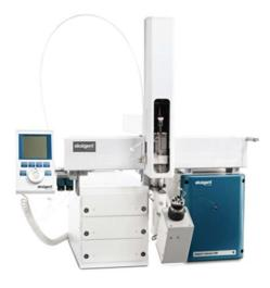
Chromatography at flow rates of 5-50 µl/min using 0.3-0.5 mm ID columns
